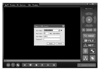
This mode allows you to remotely control your DVR via the internet or intranet using the software application.
